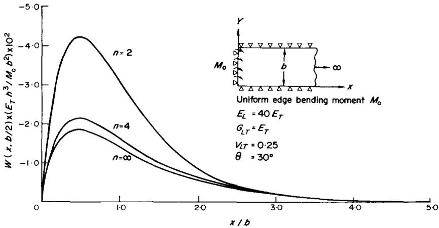
FIG. 6. Deflection along center line of  $30^\circ$  angle-ply strips under uniform edge bending moment.
