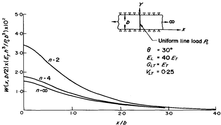
FIG. 5. Deflection along center line of 30° angle-ply strips under uniform line load.
