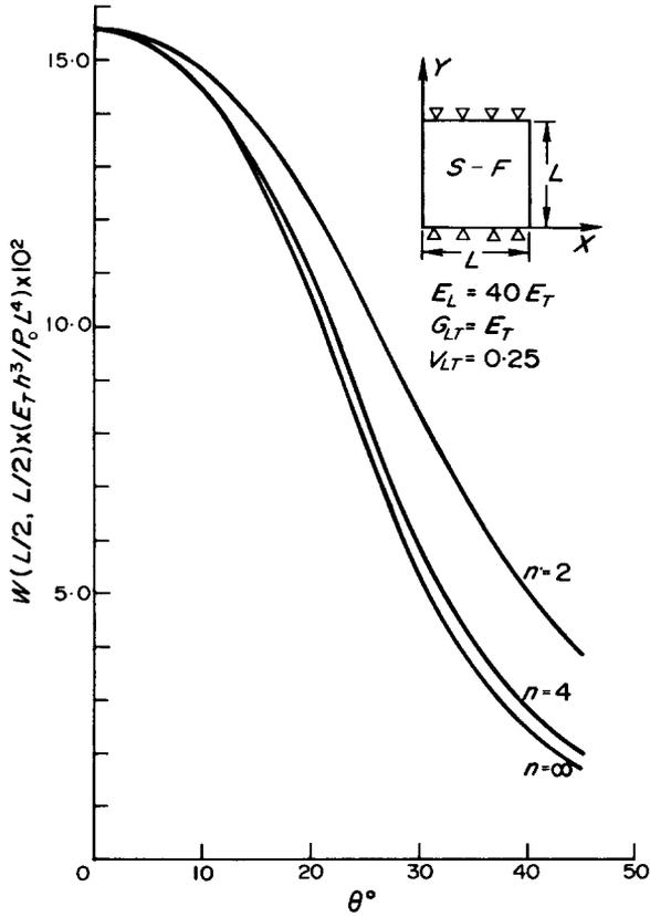
FIG. 3. Center deflection of angle-ply square plates under uniform load with simple support-free (S-F) edges vs orientation angle.
