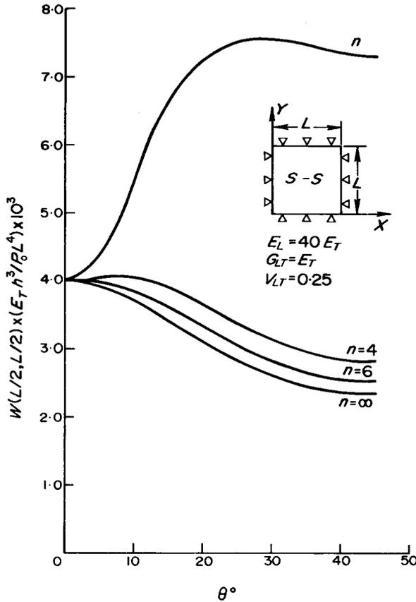
FIG. 1. Center deflection of angle-ply square plates under uniform load with simple support-simple support (S-S) edges vs orientation angle.
