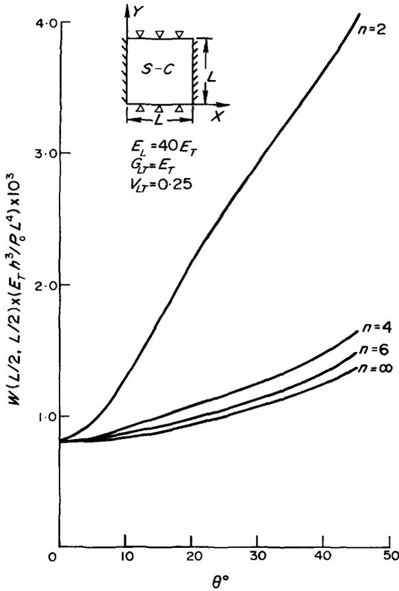
FIG. 2. Center deflection of angle-ply square plates under uniform load with simple support-clamped (S-C) edges vs orientation angle.
