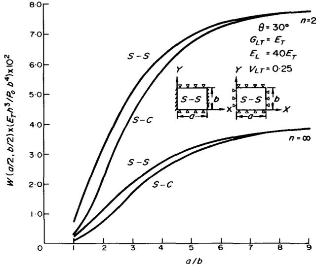
FIG. 4. Center deflection of 30° angle-ply plates under uniform load vs aspect ratio.
